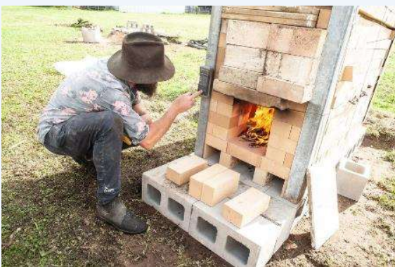
Making and firing up the smaller 'quick built' kiln. Good Job Harry!
